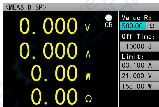
Chart 2.6.3 Constant Resistance Measurement Mode
