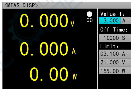
Chart 2.6.1 Constant Current Measurement Mode
