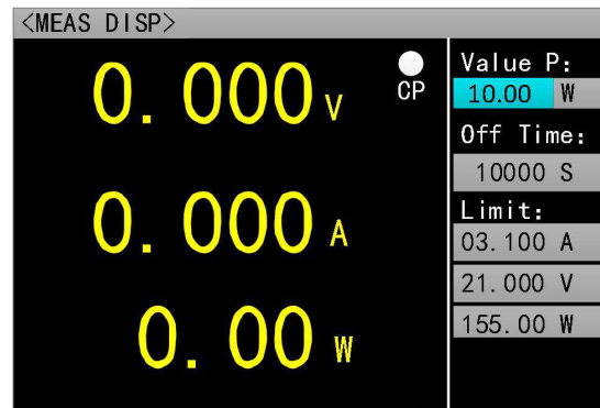
Chart 2.6.4 Constant Power Measurement Mode
